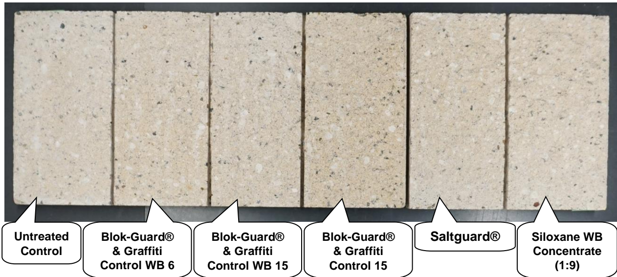
"Sandstone" Split Face CMU with Treatments
