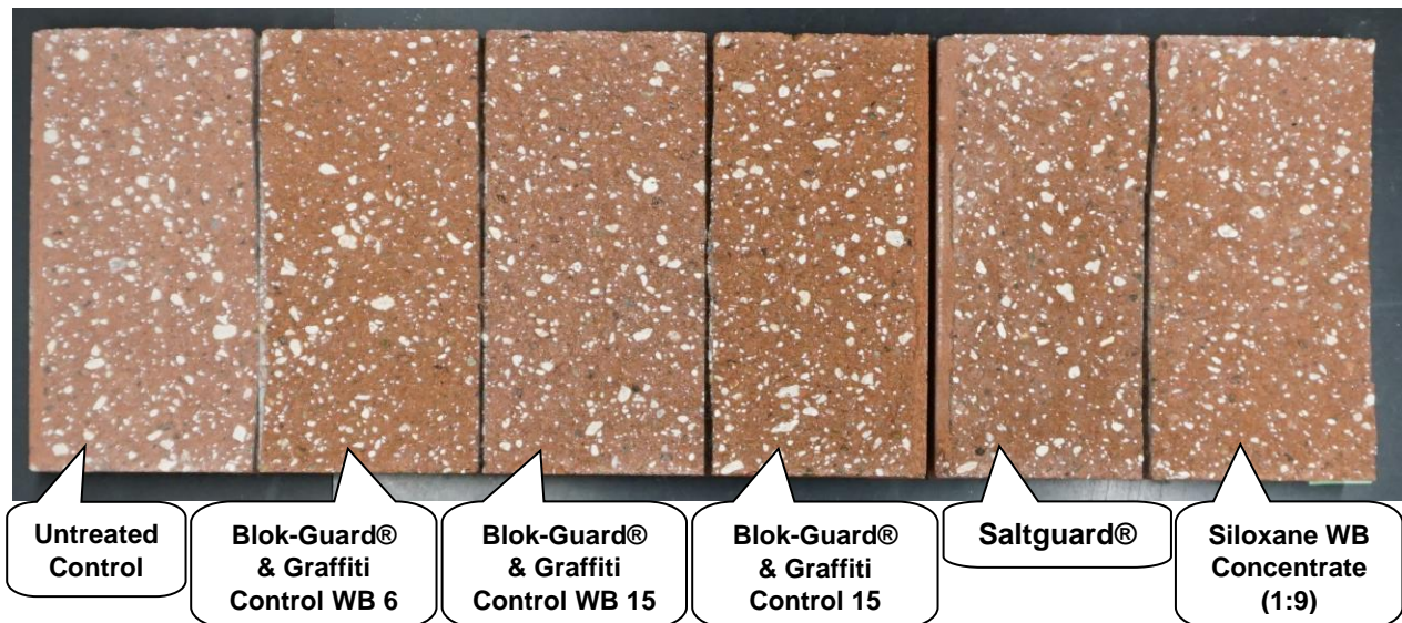
"Burgundy Red" Split Face CMU with Treatments
